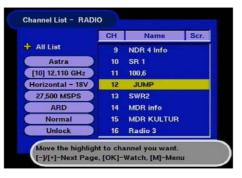
Press the button to show the programme list. A + for the main programme list or the "apple" symbol is indicated at the top left. The list can be changed by pressing the button again. Information relating to the received satellites, transponder and its frequency, the polarisation, the symbol rate, scrambling, favourite or standard programme and the parental control is
